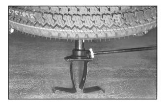
7. Place the bottom edge of the jack on the wheel blocks, separating them so that the jack is balanced securely.
